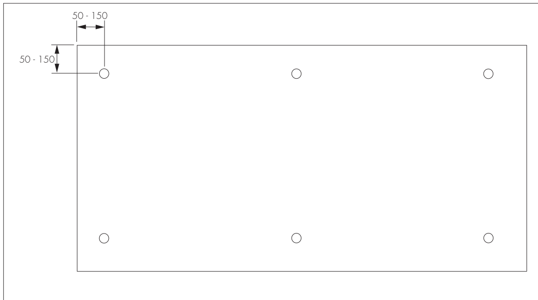
Figure 2 Fixing layout 2400 mm by 1200 mm board — minimum fixing numbers
